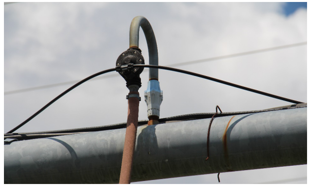
Figure 10. In this case, the pressure regulator (blue and gray piece) is attached directly to the top of the main pivot line.
