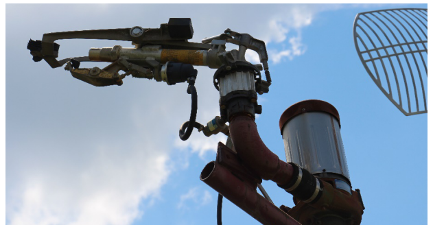
Figure 8. An end gun and booster pump. Proper operation of these components is critical for areas outside of the pivot-sprinkler coverage area.
