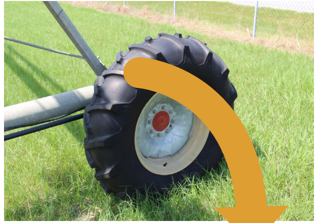
Figure 14. Cracks beginning to appear on tires. Cracks are typically due to weather wear and should be taken into consideration before the season starts. In some cases, system downtime costs more in yield than a single tire is worth.
