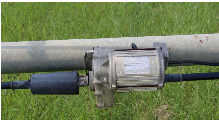
Figure 15. Gearbox on the center drive with the shroud intact around the driveline.
