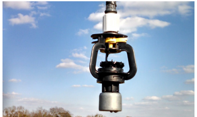
Figure 7. A new sprinkler on a drop hose. There are visible differences between new and older/worn sprinklers, which affect both appearance and operation.
