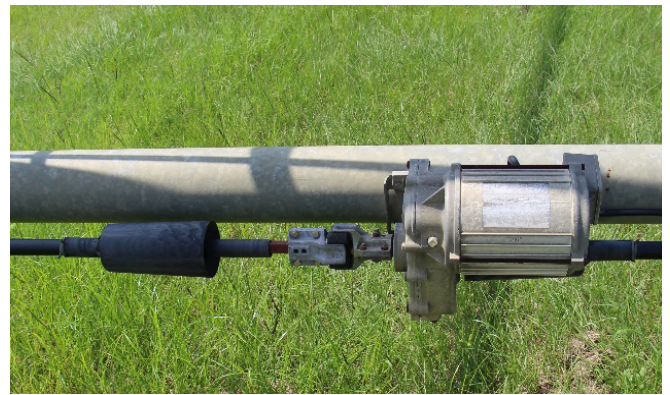
Figure 16. Gearbox with the shroud removed from the universal joint and the driveline exposed.
