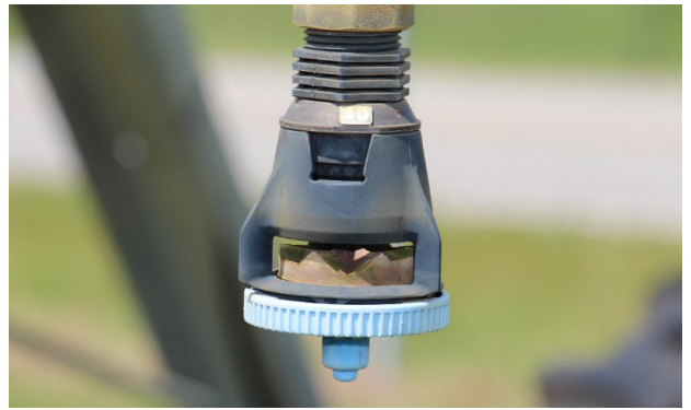
Figure 6. Visually inspect each sprinkler that does not seem to be operating correctly. Older sprinklers and components become worn due to use and weather damage, and they often need replacing to ensure maximum coverage and efficiency.
